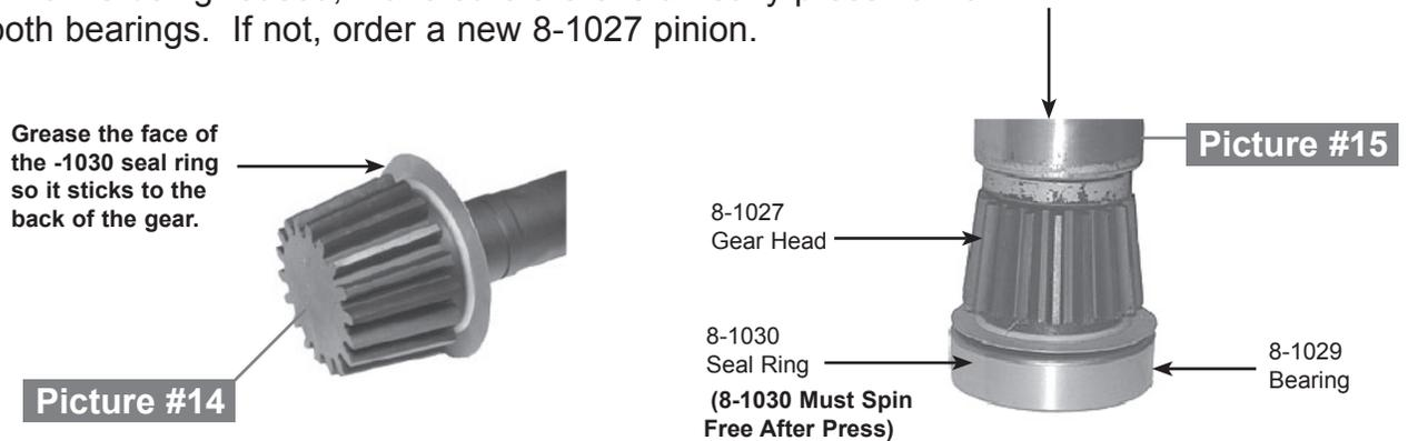
**Step 16** 8-1027, 8-1030, 8-1029 press into 8-1031 - NOTE: It is highly recommended that the internal cavity of the 8-1031 bearing housing be totally packed with grease in order to protect the bearings from coolant penetration.
